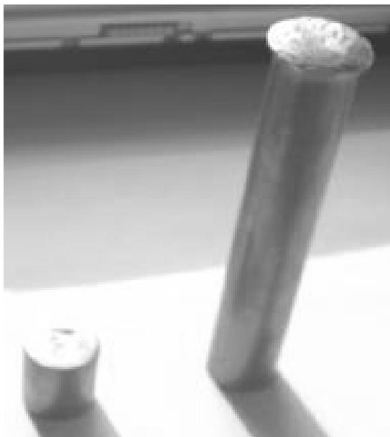
Fig. 4: Lower or pile die (left) and upper or trussel die (right) after hand-striking in an experiment by Di Hu.<sup>6</sup> The upper die shows mushrooming due to the impact of the hammer, while the lower die shows no such deformation after equal use. The same effect was earlier reported by Sellwood, whose first upper die split. Surviving ancient dies show the same effect.
